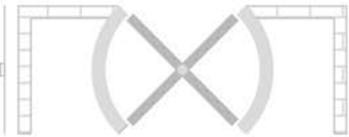
Enclosure set back within a wall recess
